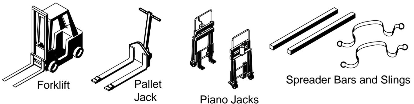
If possible, transport the Liebert DS with a forklift or pallet jacks. If that is not possible, use a crane with belts or cables, slings and spreader bars.
