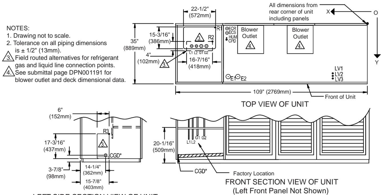
\* Field pitch Condensate Drain line a minimum of 1/8" (3.2 mm) per foot (305 mm). All units contain a factory installed condensate trap. Do not trap external to the unit. Drain line may contain boiling water. Select appropriate drain system materials. The drain line must comply with all local codes.
