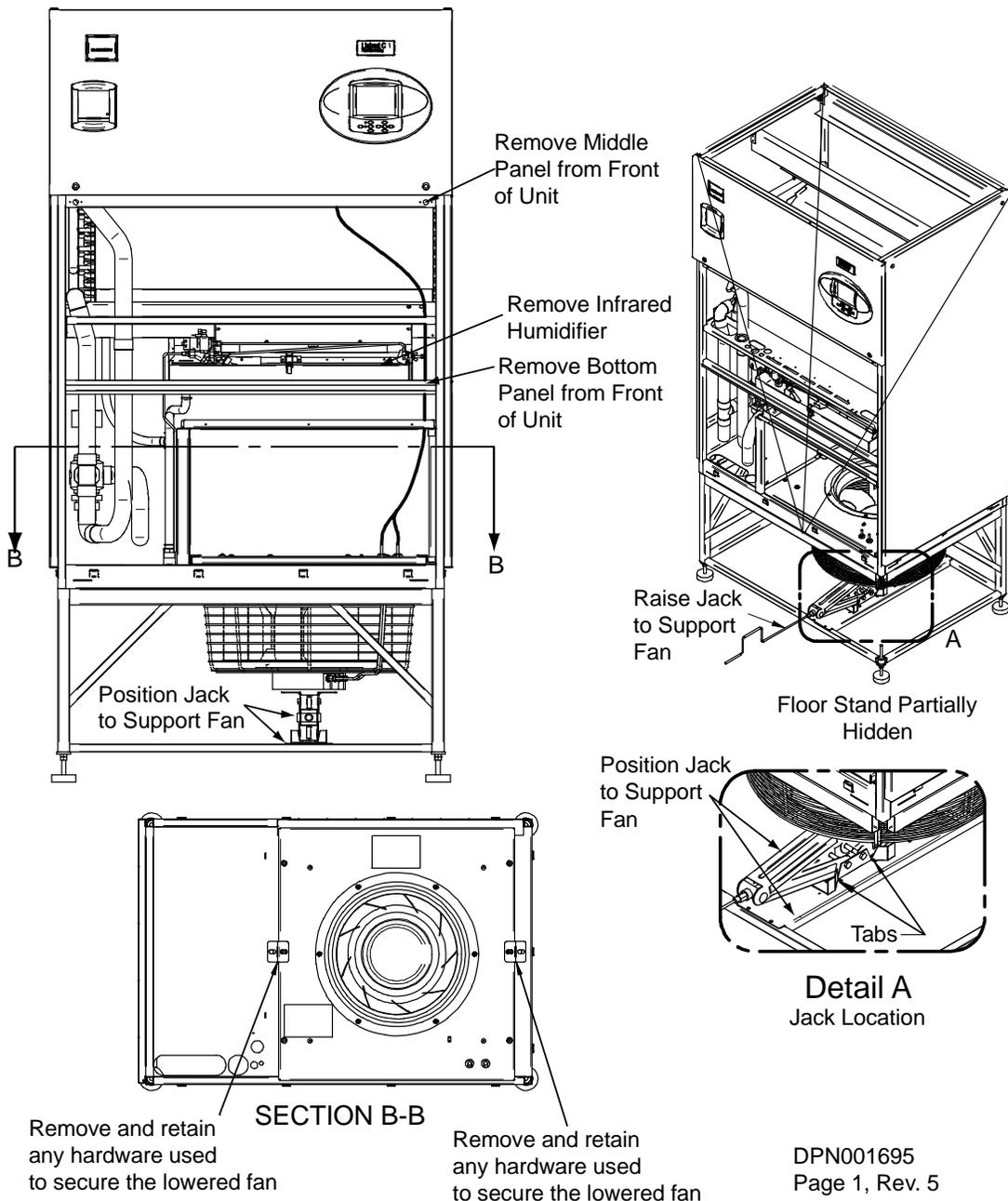
6. Insert a field-supplied fan removal device under the fan module. The fan removal device should rest securely on the front and rear frame channels.
