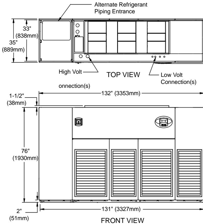
**Note:** Front air return unit shown. For rear return unit, in addition to front service area shown, also include 25" (635mm) on one side of unit for access to rear return filter box. See DPN001196, Figure 30.
