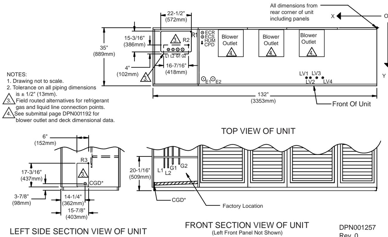
Table 57 Piping data—upflow, air-cooled 105kW (30 ton), all
