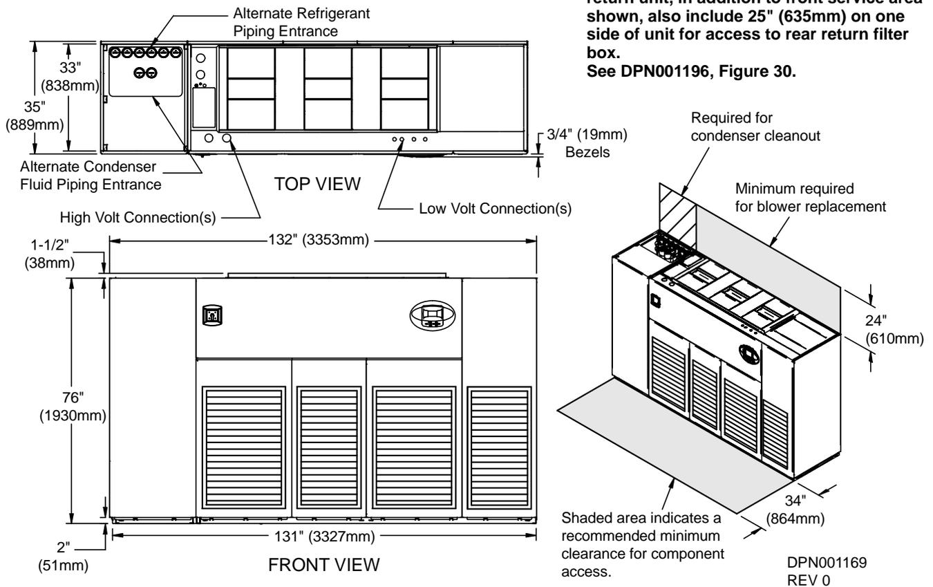
**Note:** Front air return unit shown. For rear return unit, in addition to front service area shown, also include 25" (635mm) on one side of unit for access to rear return filter box. See DPN001196, Figure 30.
