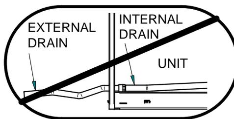
THESE ARE EXTERNAL TRAPS ALSO, ALTHOUGH UNINTENTIONAL. LINES MUST BE RIGID ENOUGH NOT TO BOW OVER TOP OF OTHER OBJECTS.
