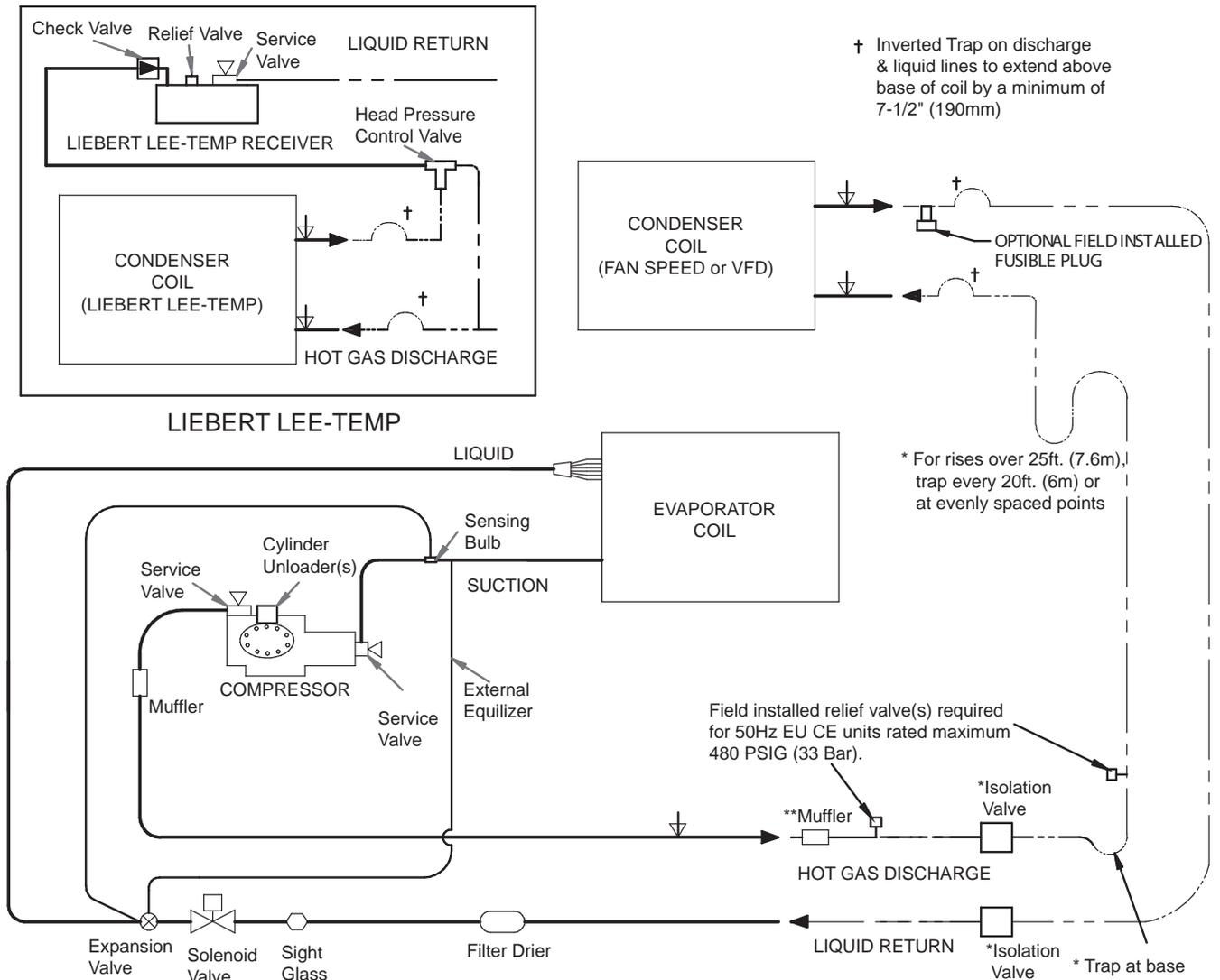
† Inverted Trap on discharge & liquid lines to extend above base of coil by a minimum of 7-1/2" (190mm)
