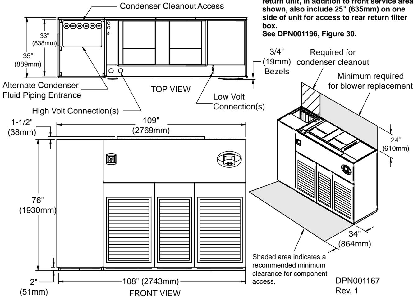
**Note:** Front air return unit shown. For rear return unit, in addition to front service area shown, also include 25" (635mm) on one side of unit for access to rear return filter box. See DPN001196, Figure 30.
