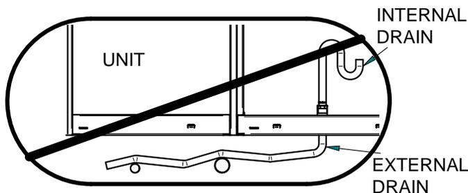
THESE ARE EXTERNAL TRAPS ALSO, ALTHOUGH UNINTENTIONAL. LINES MUST BE RIGID ENOUGH NOT TO BOW OVER TOP OF OTHER OBJECTS.
