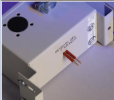
*Liebert Liqui-TECT 410 sensor offers leak detection at critical points under a raised floor. Two corrosion-resistant gold-plated probes detect moisture and immediately signal the monitoring system, allowing fast action to be taken before mission-critical equipment is damaged.*
