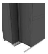
Two wheels in the middle of the rack help the smooth movement of the rack. However, the weight is mainly supported by the telescopic rails. Two hasps fixed on each telescopic rail complete the system, setting the rack in its mid position.
